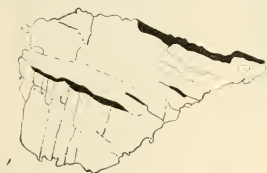
FIG. 4.—Natural Widmanstätten figures brought out by burnishing.
